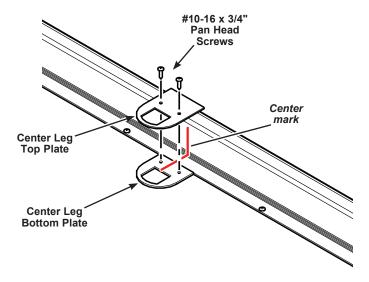
5. Place the center leg spacer flush against the center rail and centered over the center mark as shown.
