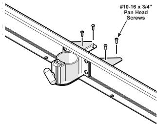
10. Insert, attach and secure a leg into the pocket assembly using the same procedure as the other legs.
