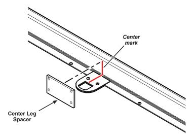
6. Tilt the straight corner pocket assembly to fit the bottom of the shoe into the square hole of the center leg bottom plate.
