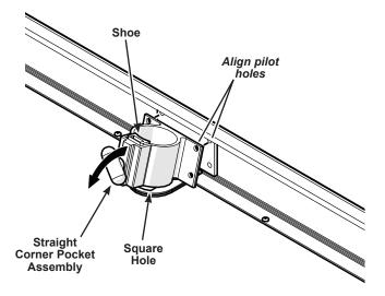
7. Using the aligned sets of pilot holes in the straight corner pocket assembly and center leg spacer as a guide, drill four 1/4" (6 mm) holes straight through the center rail.
